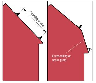
The tables are based on fixings c/c 1200 mm. Distance table for snow guards according to SS 83 13 35:2012 with snow zones according to BFS 2015-6-EKS 10 and form factor according to Eurocode SS-EN 1991-1-3. Loads on load-bearing elements – Parts 1-3: General loads – Snow load.
